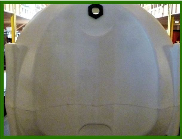
Water tank for NSHC at FS work shop before transport to NSHC. Drilled and installed valves on 1425 gallon tank. One 3-inch inlet valve, one 1 ½-inch outlet valve.
