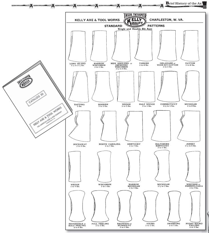
Figure 9—Some standard patterns manufactured by True Temper Kelly in 1925.
