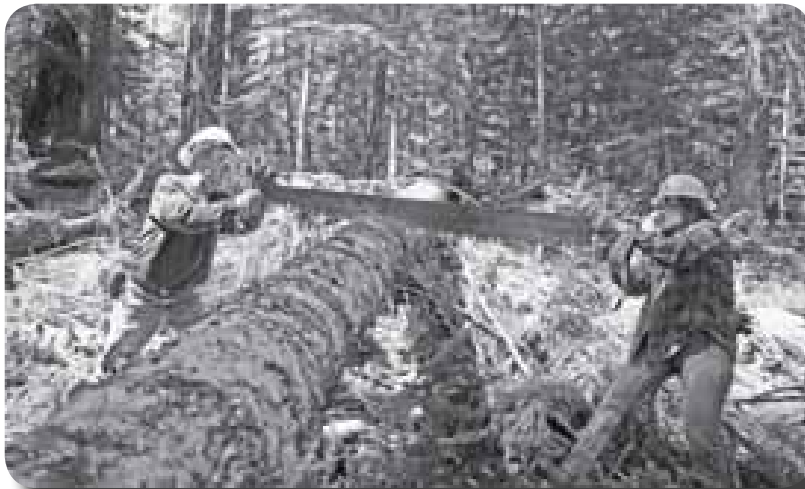
Joe and Cindy Chenier working on a windfall with the two-man crosscut saw.
